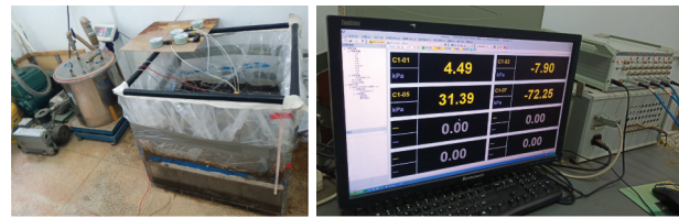
FIGURE 4: Rapid sludge dewatering system with a vacuum negative pressure load at the bottom of the full section. (a) Schematic diagram of test model system. 1, vacuum pump; 2, gas-water separator; 3, electronic scale; 4, valve; 5, vacuum gauge; 6, connecting pipe; and 7, model box. (b) Test model pictures.
