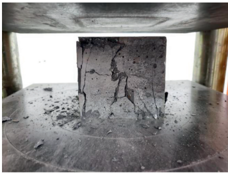
FIGURE 8: Failure condition of compressive specimens.
