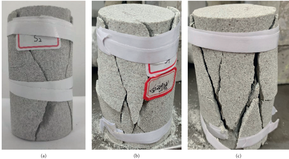
FIGURE 6: Macroscopic failure modes of rock samples on different moisture conditions during the uniaxial compression test. (a) Dry state. (b) Natural state. (c) Water-saturated state.
