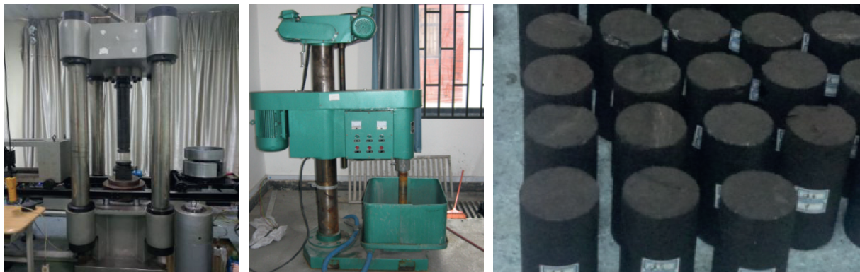
FIGURE 2: Sketch of the preparation of argillaceous sandstone, coal, and silty sandstone.
