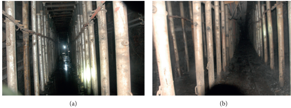
FIGURE 10: Roadway in the mining-induced advanced abutment pressure area of the fracturing area.
