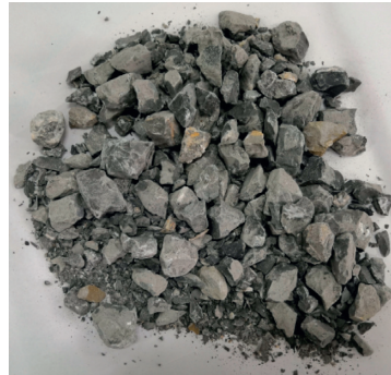
FIGURE 7: The crushed rock particles after compaction.
