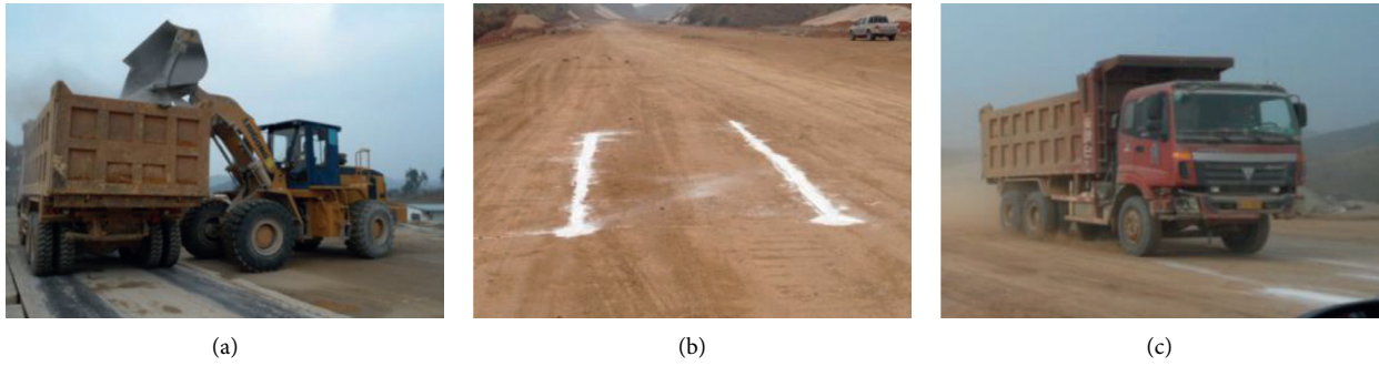
FIGURE 5: Preparation and testing process: (a) truck rear axle weighing, (b) marked position of the sensor, and (c) the truck passing over the sensor.
