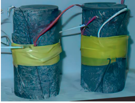
FIGURE 1: Rock failure under the uniaxial compression test.
