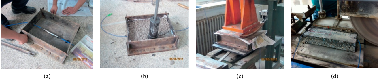
FIGURE 4: Beam-specimen fabrication procedure. (a) Sensor positioning; (b) mixture filling; (c) molding; (d) cutting.
