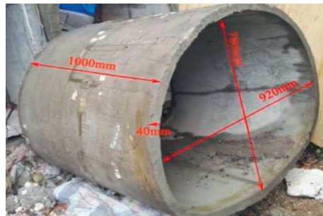
FIGURE 10: Oval tunnel lining model.
