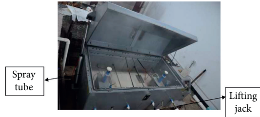
FIGURE 1: Inner structure of salt spray corrosion test chamber.
