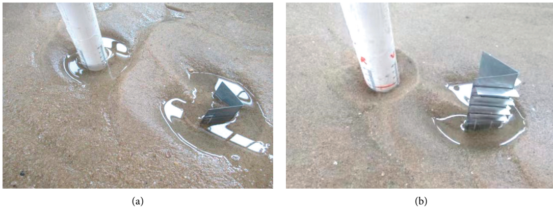
FIGURE 4: Characteristic map of scour pit: (a) wingless plate; (b) with wing plate.
