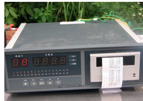
FIGURE 2: The instrument for recording and printing temperature data.
