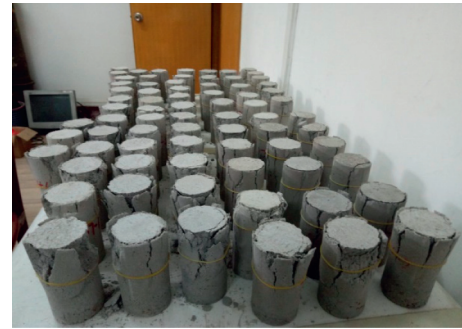
FIGURE 4: Specimen deformation and failure.
