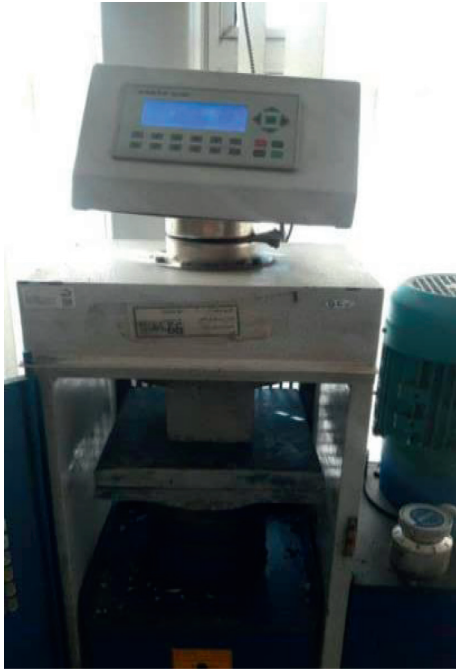
FIGURE 2: Hydraulic test Jack.
