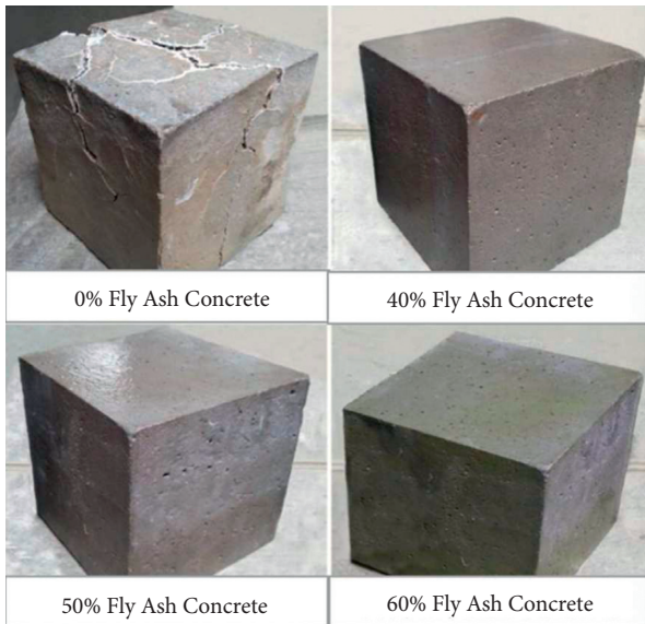
FIGURE 11: Concrete cubes after exposure to 10 wt.% sodium sulfate solution, reproduced from [90], a paper published in an open access journal.
