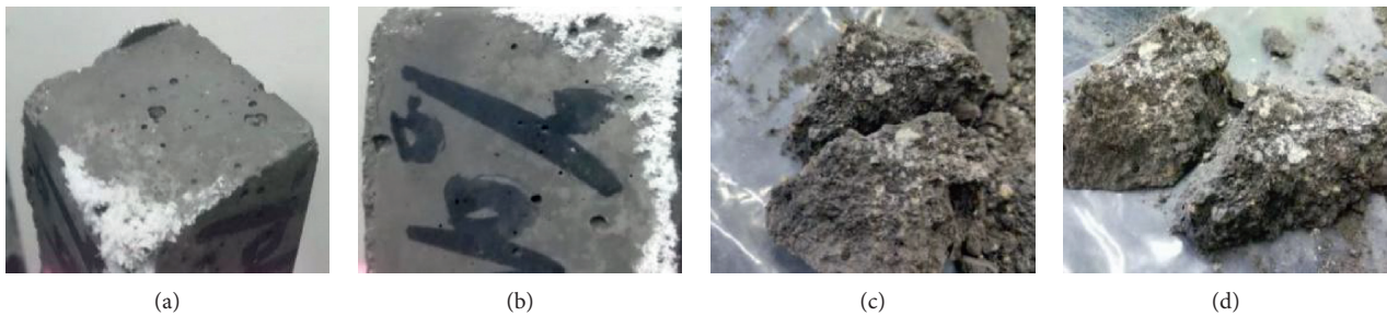
FIGURE 16: Internal and external characteristics of the M7S10 and M7G10 test specimens. (a) External apparent morphology of 28 d of M7S10; (b) external apparent morphology of 28 d of M7G10; (c) internal apparent morphology of 28 d of M7S10; (d) internal apparent morphology of 28 d of M7G10.
