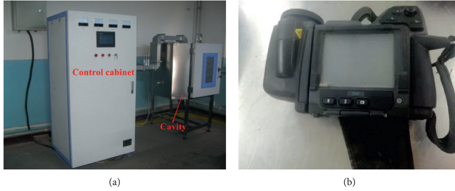
FIGURE 5: Test instrument(a) Industrial microwave oven. (b) Infrared temperature measuring meter (FLIR).
