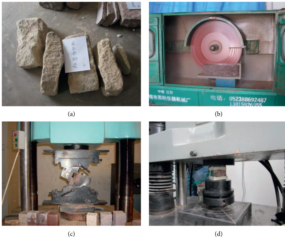
FIGURE 2: Rock mechanics experiment: (a) primary sample, (b) sample cutting, (c) rock shear test, and (d) uniaxial compression experiment.
