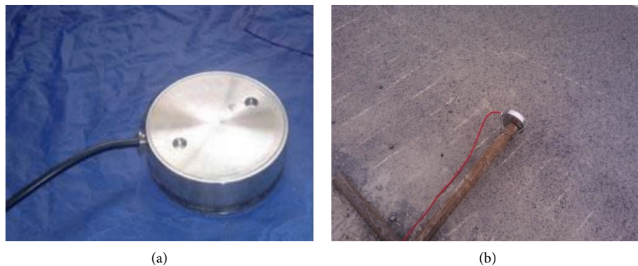
FIGURE 2: Installation and layout of the earth pressure boxes. (a) XB-150 double-membrane earth pressure cell. (b) Site of earth pressure box installation.
