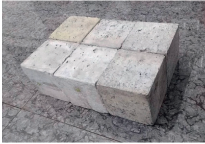
FIGURE 1: Processed concrete samples.
