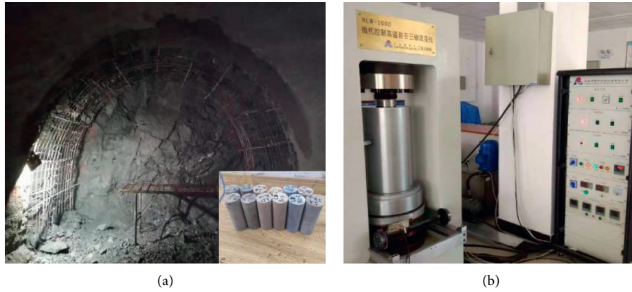
FIGURE 5: Experimental process of rock mass in the station. (a) Rock specimen collection and preparation. (b) Triaxial experimental instrument.
