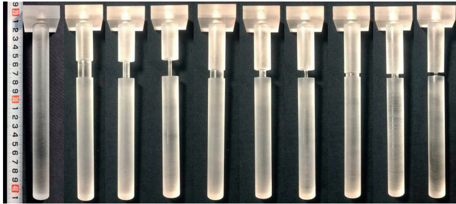
FIGURE 7: Intact pile and shallow necking piles.
