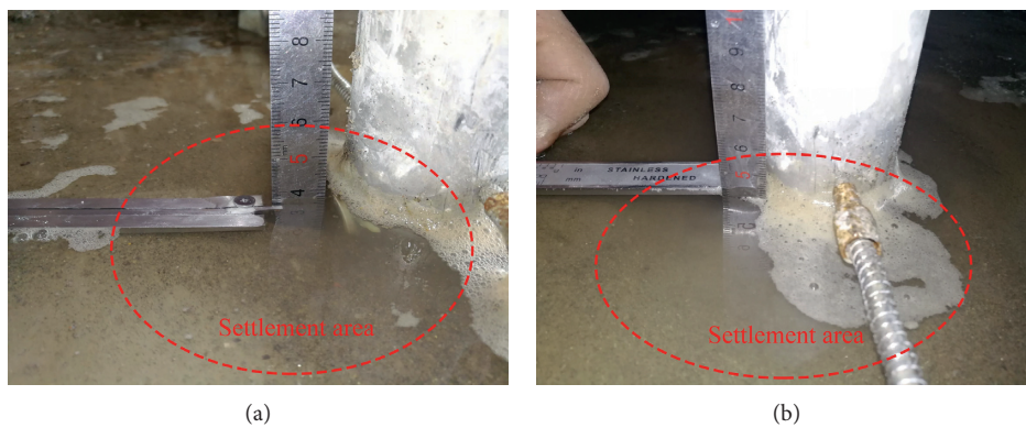
FIGURE 17: Settlement with different cycles around pile in case 6: (a) N=1000 cycles; (b) N=5000 cycles.
