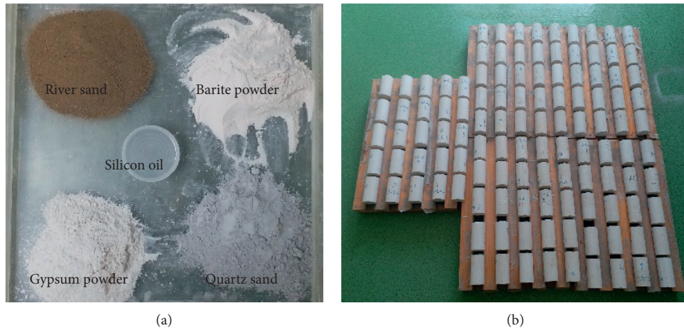
FIGURE 4: Similar materials. (a) Components of similar materials and (b) standard specimens of different proportions.
