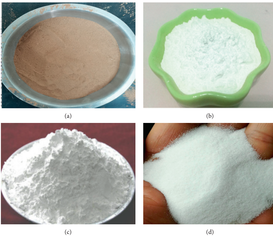
FIGURE 2: Comparison of test materials. (a) Sandy silt. (b) 400 mesh quartz flour. (c) 2500 mesh quartz flour. (d) 40–70 mesh quartz sand.
