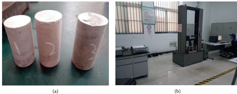
FIGURE 7: Rock samples preparation and test procedure: (a) mudstone samples and (b) test procedure.
