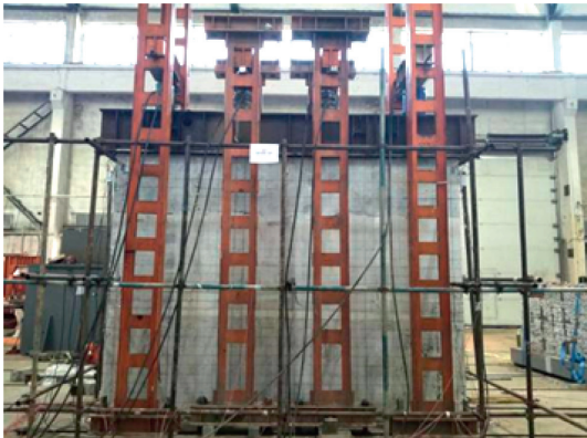
FIGURE 4: The loading device of the compressive experiment.
