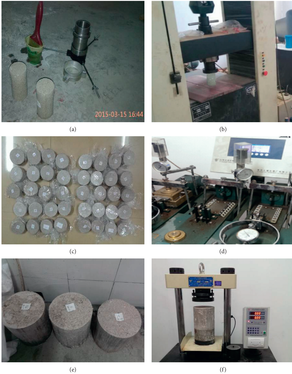
FIGURE 2: Parameter tests of similarity material for surrounding rock. (a) Elastic modulus test specimen. (b) Elastic modulus test. (c) Direct shear test specimens. (d) Direct shear test. (e) UCS test specimen. (f) UCS test.
