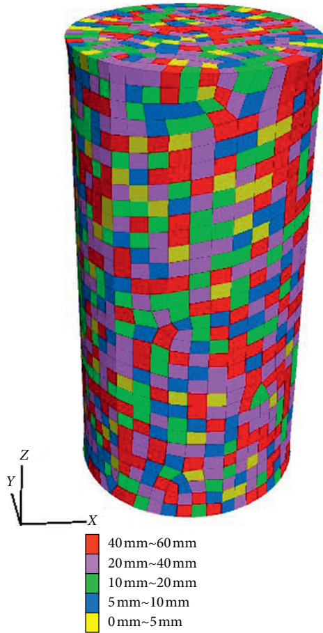
FIGURE 8: A schematic diagram of a triaxial numerical specimen.
