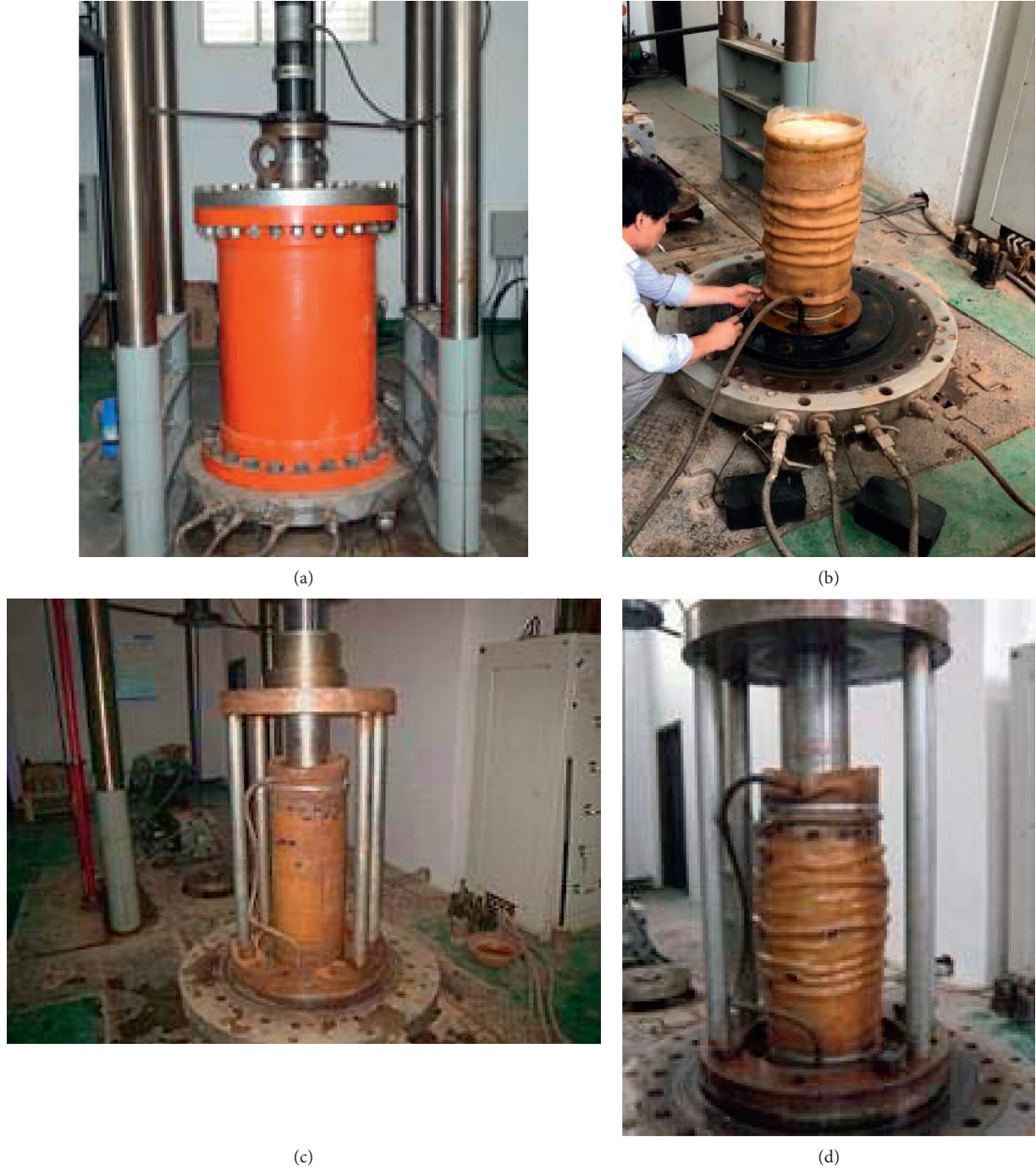
FIGURE 4: Large-scale triaxial test of coarse-grained materials: (a) laboratory apparatus; (b) installation sample; (c) before the test; (d) after the test.
