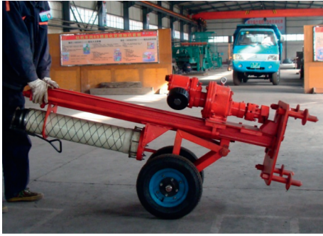
FIGURE 3: Roadway floor anchor cable drilling rig.
