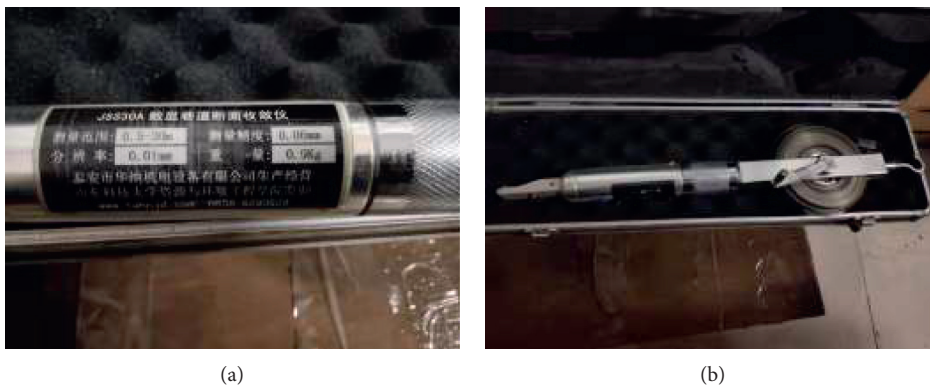
FIGURE 15: JSS30A digital display roadway section convergence instrument.
