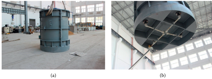
FIGURE 2: (a) The model box. (b) Model box drainage system.
