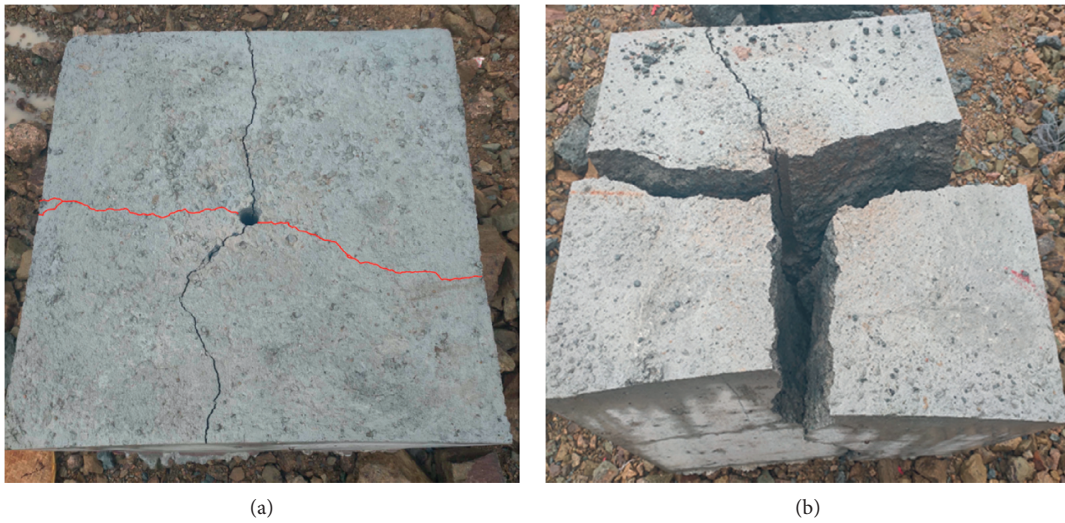
FIGURE 7: Damage and crack propagation of single-hole blasting: (a) conventional blasting; (b) multidirectional shaped charge blasting.
