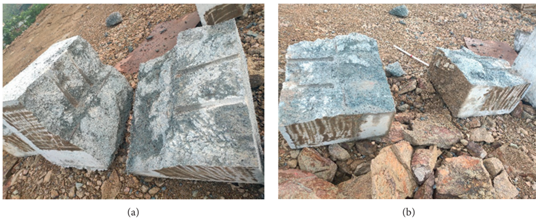
FIGURE 8: Damage and crack propagation of dual-hole blasting: (a) conventional blasting; (b) multidirectional shaped charge blasting.
