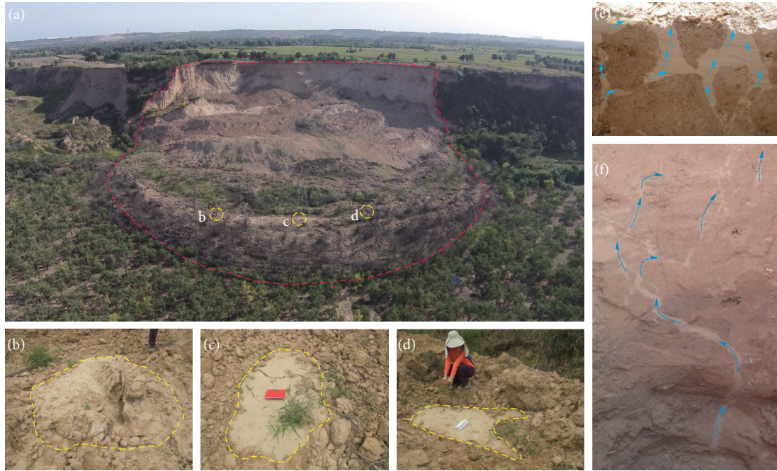
FIGURE 1: A typical Jingyang landslide and some liquefaction phenomena. (a) Drone view of a typical Jingyang landslide. (b), (c), and (d) Photographs of some traces of sand boiling from liquefaction. (e) and (f) Profiles of the sand boil at (d) obtained by trenching.
