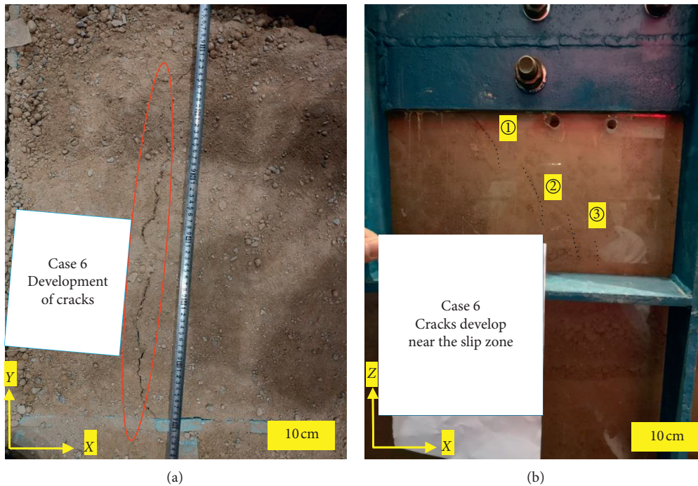
FIGURE 13: Schematic diagram of cracks on the left and right sides of the slope. (a) Lateral cracks on the right-side slope of 0.6 g. (b) Diagonal crack on the left-side slope of 0.6 g.
