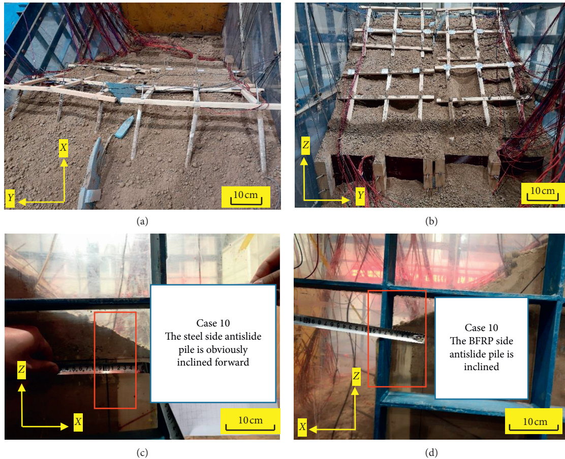
FIGURE 14: Deformation of anchor rod and antislip pile. (a) 1.4 g bolt exposed. (b) 1.4 g slope flow phenomenon. (c) 1.4 g left slope antislip pile tilt. (d) 1.4 g right slope antislip pile tilt.
