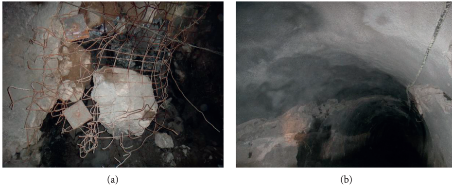
FIGURE 1: Ground pressure deformation and failure map of Jinchuan No. 2 mining area. (a) Failure of the supporting system. (b) Failure of the roadway.
