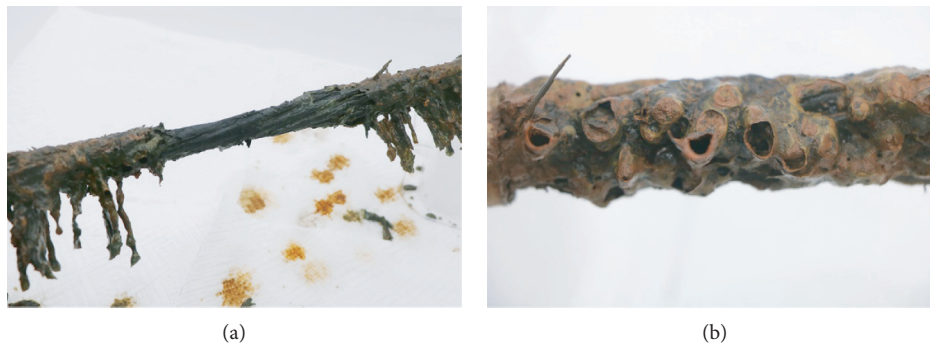
FIGURE 3: Morphology of corroded anchor sample. (a) Loose and flaky corrosion product; (b) distributed holes.
