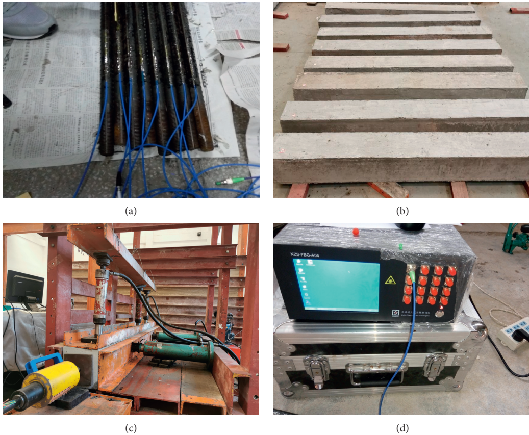
FIGURE 2: Bolt drawing test. (a) Grating force-measuring bolt. (b) Simulating surrounding rock block. (c) Bolt drawing test platform. (d) Fiber grating demodulator.
