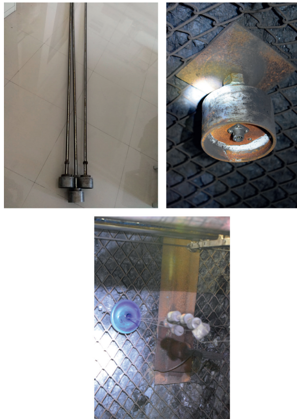
FIGURE 7: Force-measuring bolts and multipoint displacement meters of the mining roadway.
