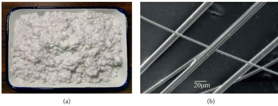
FIGURE 1: Appearance and micrograph of ceramic fibers.
