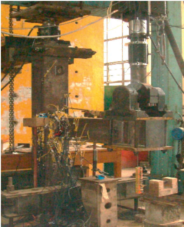
FIGURE 8: Test setup of T-stub connection for static behavior.
