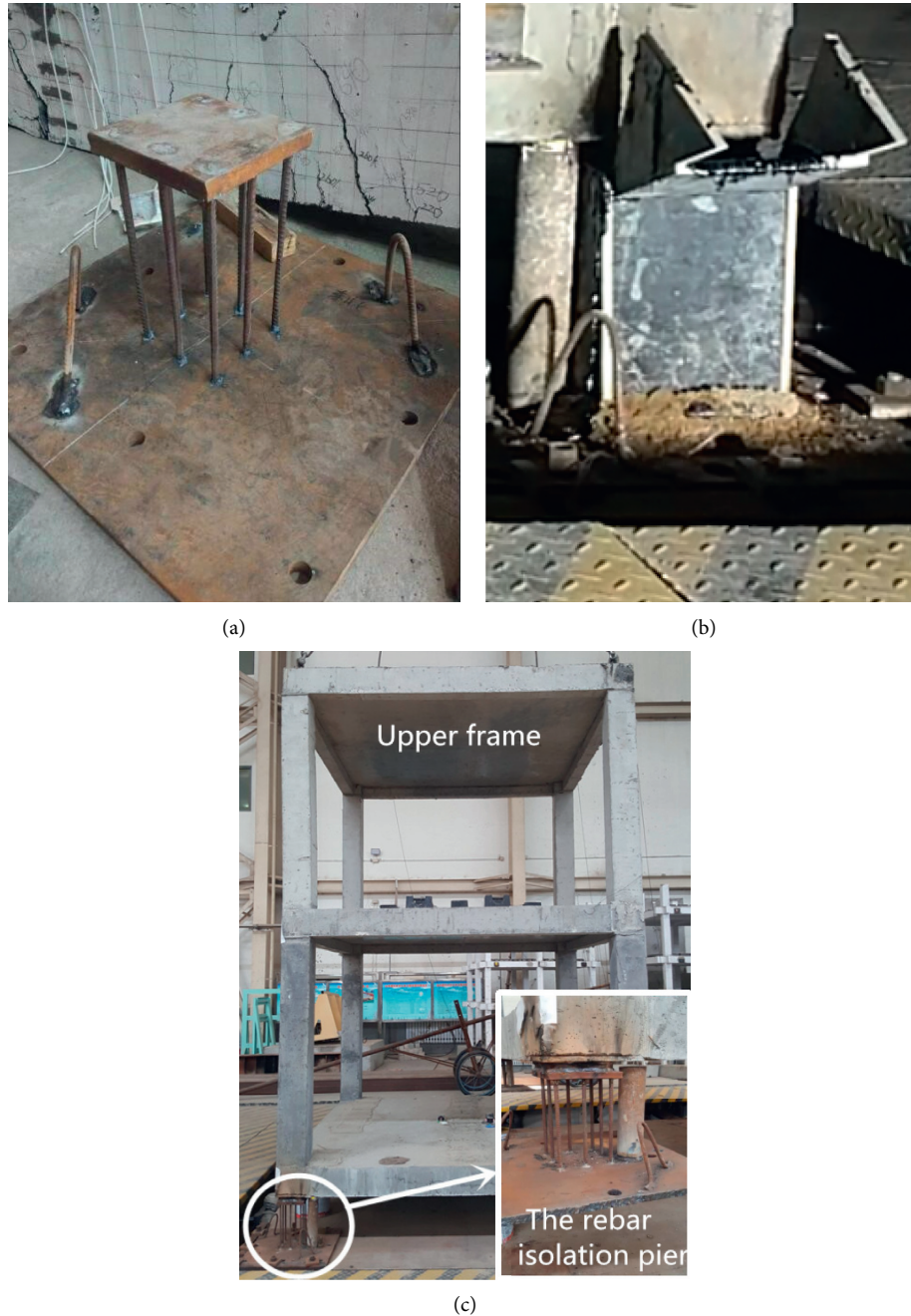
FIGURE 5: Real object of the rebar isolation pier: (a) rebar isolation pier without asphalt ointment, (b) rebar isolation pier with asphalt ointment, and (c) installed experimental model.
