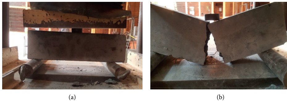
FIGURE 6: Flexural strength testing. (a) Flexural strength test setup. (b) Failure mode of concrete under bending.
