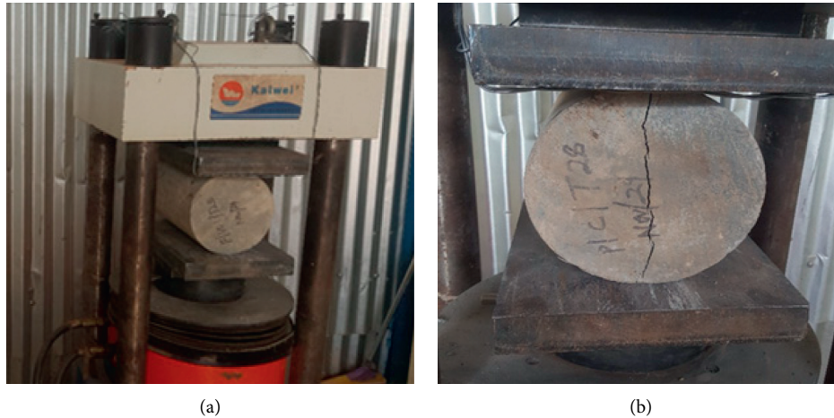
FIGURE 5: Splitting tensile strength testing. (a) Splitting tensile strength test setup. (b) Failure mode of concrete under splitting tension.
