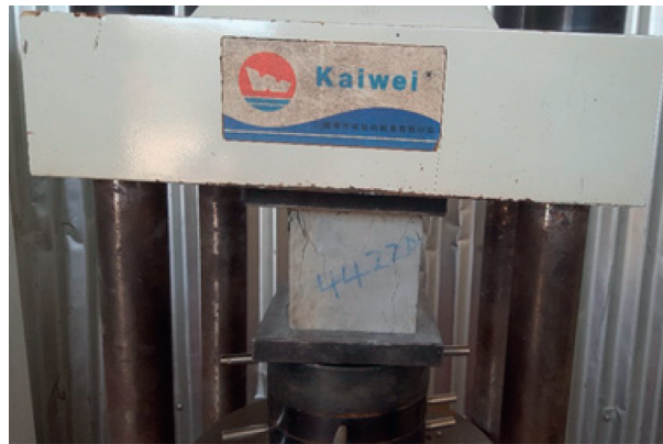
FIGURE 4: Compressive strength test setup.
