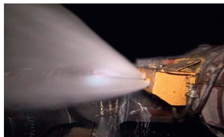
FIGURE 9: Field application diagram of the shearer external spray unit.
