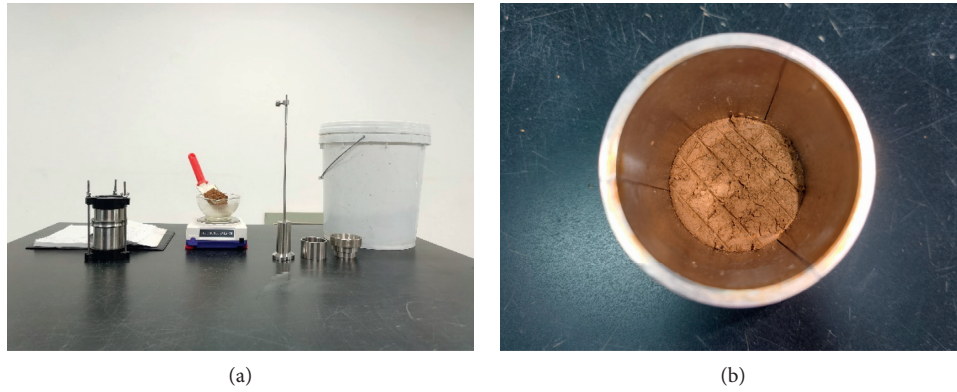
FIGURE 3: The procedures for preparing triaxial samples. (a) Sample weight. (b) The top of each layer was scarified prior to adding the next layer.
