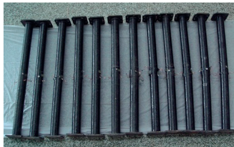
FIGURE 7: The C-CF-CFRP-ST specimens after loading.
