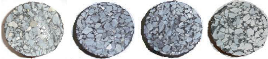
FIGURE 3: R-OGFC specimen profile (the content is 0, 1%, 2%, and 3%).
