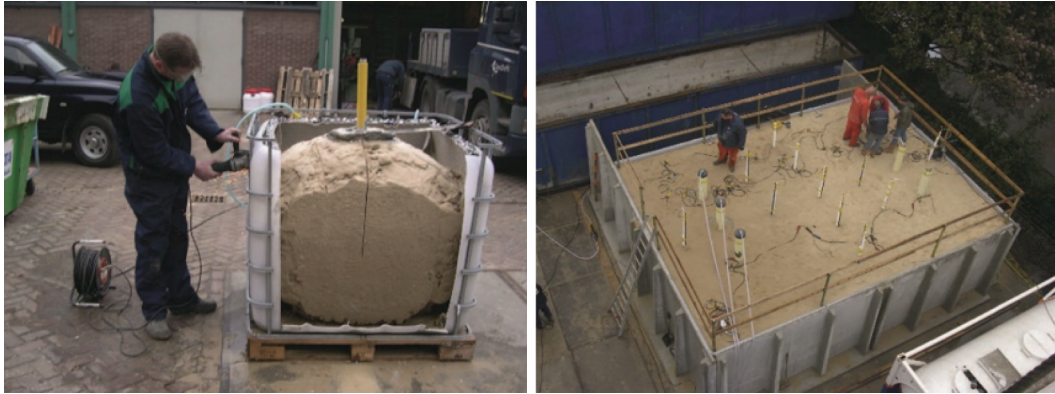
FIGURE 9: A wide range of experimental devices for biological cementation ( 1 \text{ m}^3 and 100 \text{ m}^3 ) [32].
