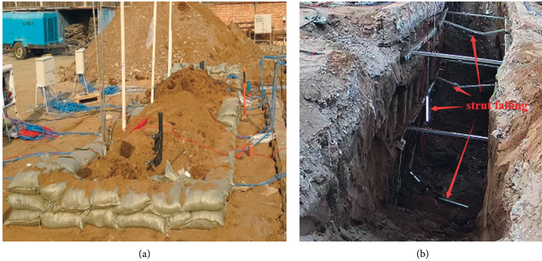
FIGURE 8: Simulation of test conditions. (a) Pit side loading. (b) Strut falling.
