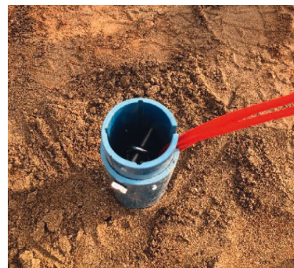
FIGURE 4: Burying the inclinometer.
