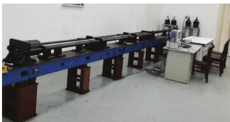
FIGURE 3: SHPB experimental equipment.
