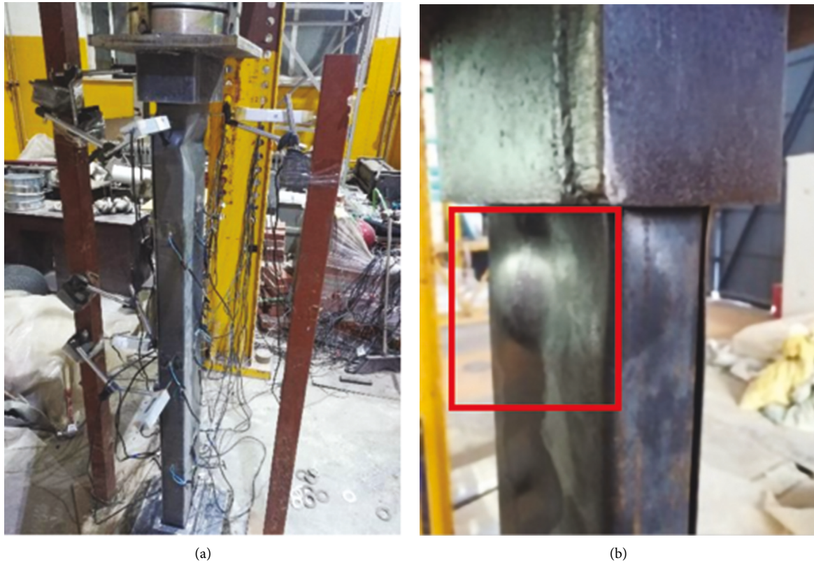
FIGURE 9: Damage of the specimen Z200-3.0-k. (a) Overall. (b) Local buckling.
