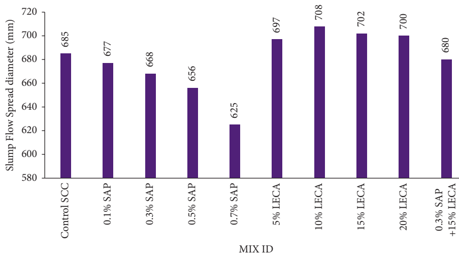
FIGURE 7: Slump flow spread diameter of all SCC mixes.
